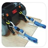
Fitting the rear restraint
