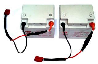
The positive (+) terminal is connected with a RED wire.
