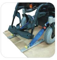
Fitting the front restraint
